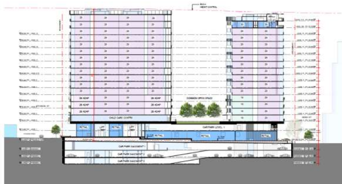
Figure 3 Section showing compliance with the 60m maximum height limit
